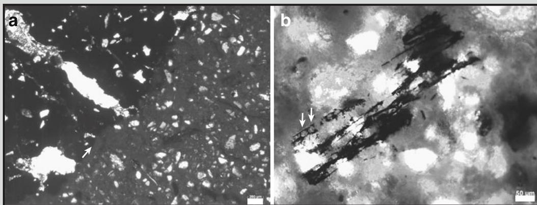
**Figure 6.** Thin section images taken from the chest concretion preserved in “Willo.” In (a), the wall of the concretion is shown to be composed of sand grains (light colored spots) cemented together by iron-rich minerals (darker material). In (b), a small piece of plant fossil from the wall of concretion is shown surrounded by sand grains. Images modified from Cleland and others (2011: figs. 3a and b).
